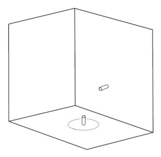
Remove the basin, install the waste pipe either at the height of the entrance horizontally, or within the perimeter of the basin vertically.
