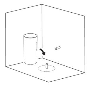
Re-position the basin into the fixing area, connect the waste. Before putting the basin into the final position, pour some water into the basin to ensure there are no leaks from the waste.
